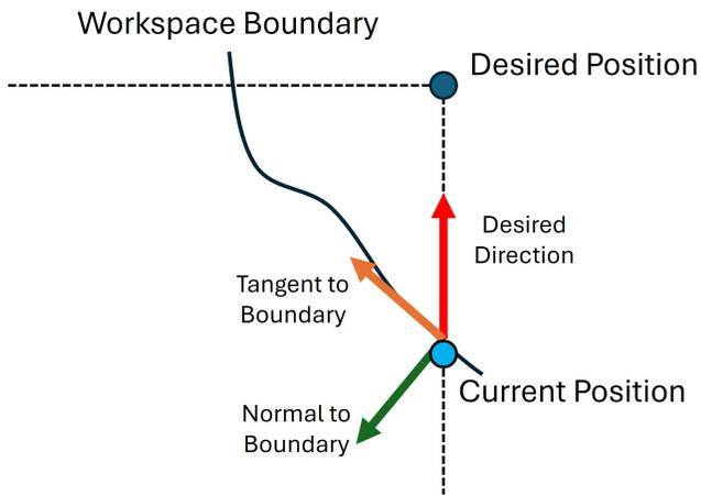
Fig. 4: The visualized method for traversing along the unknown workspace boundary by using the method of the 7th (or 4th) smallest eigenvalue
