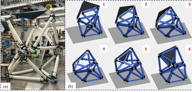
Fig. 2: (a) Solar panel array composed of six triangles and the solar panel. (b) Simulation of solar panel configuration for the robotic truss showcasing its motion that can reorient the solar panel in the direction of most sunlight.
