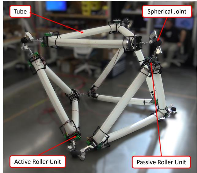
Fig. 1: An octahedron unit of the isoperimetric truss robot with its main subsystems highlighted: the inflated tubes, the spherical joints, and the active and passive roller units.
