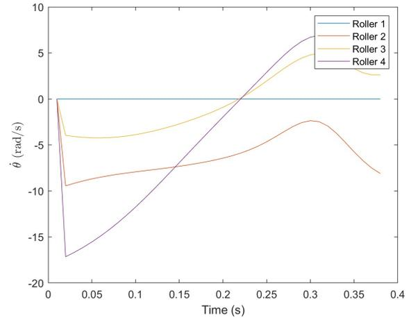
Fig. 3: Plot showing the roller velocities of each motor, including Roller 1's constrained motion
