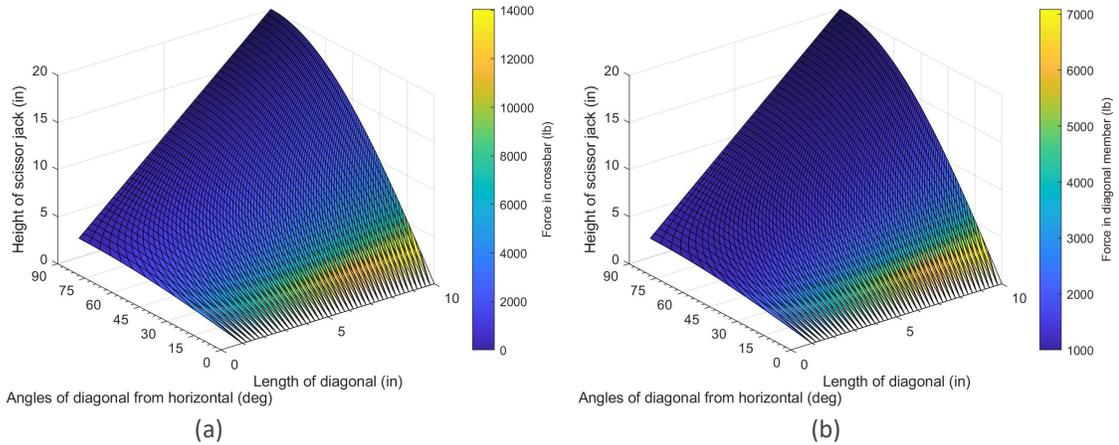
Figure 3. Surface plots show the force in the (a) crossbar and (b) diagonal member as a function of height and operating angle.
